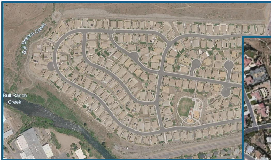
Above: New subdivision allowing natural topography and off-site features to inform the design. Roadways provide logical connectivity within the neighborhood and to the outside world.
